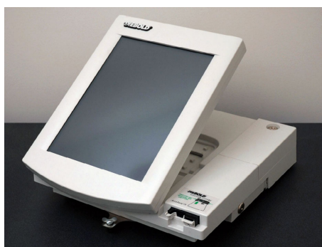
Fig. 1: The Diebold AccuVote TS Direct Recording Electronic voting machine. [68]
